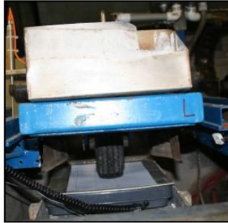
b) Contact Area Print Process
